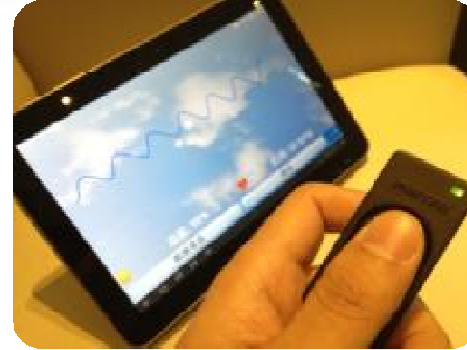
Pulse Oximetry Done (57x27x14.5mm, 15g)
